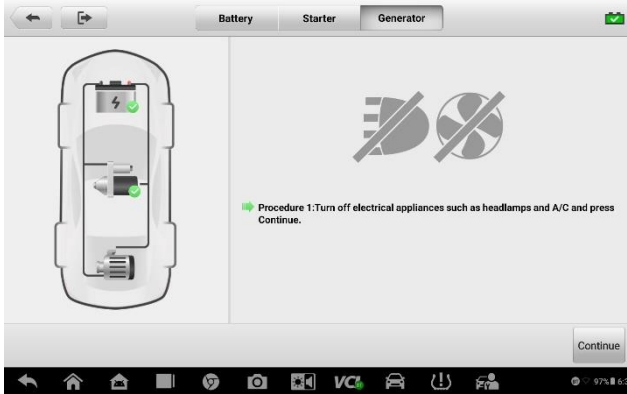
Figure 7-11 Sample Generator Test Screen
