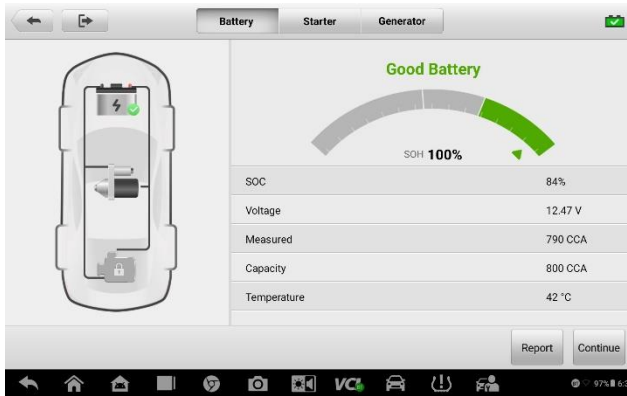
Figure 7-7 Sample Battery Test Results Screen
