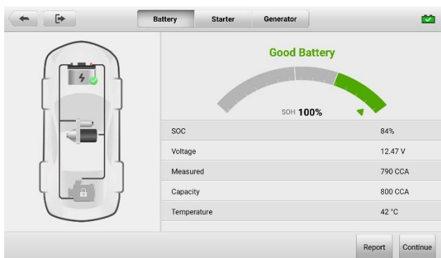
Figure 6-7 Battery Test Results Screen
