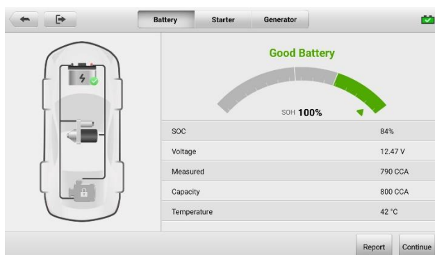
Figure 6-7 Battery Test Results Screen
